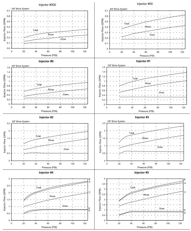
A) Total Flow, 3/8" Brine System B) Total Flow, 1/2" Brine Line C) Rinse D) Brine Draw, 3/8" Brine System E) Brine Draw, 1/2" Brine Line NOTE: All data taken with 2310 Safety Brine Valve and 500 Air Check
