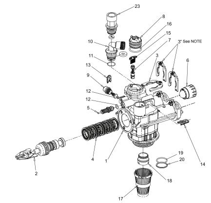
NOTE: Installers are responsible for securing the plastic H Clips (p/n 40576 red clips) when attaching connectors. The red clips will break if you attempt to force into position without fully inserting the connector into the body. If the connector is inserted properly the red clip insertion path will be clear.
